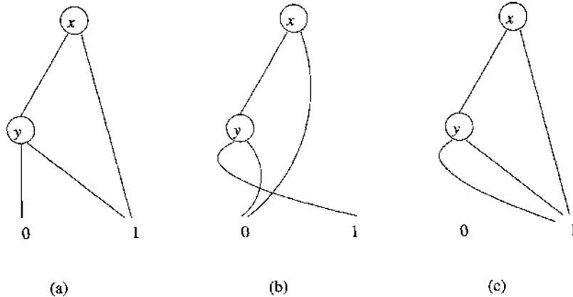
Figure 12.33: Constructing the BDD for a logical OR
