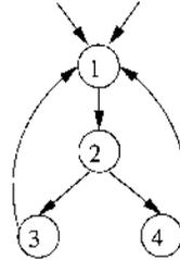
Figure 9.46: Two loops with the same header
