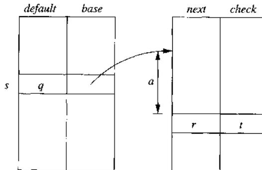
Figure 3.66: Data structure for representing transition tables
