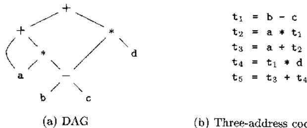
Figure 6.8: A DAG and its corresponding three-address code
