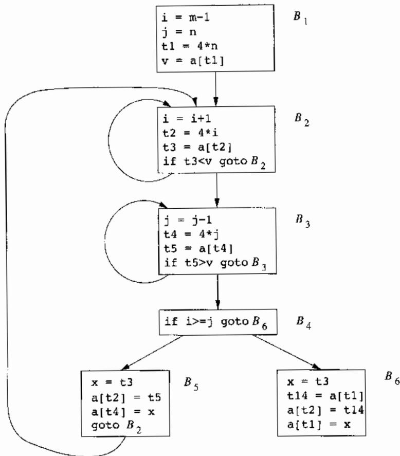
Figure 9.5:  $B_5$  and  $B_6$  after common-subexpression elimination
