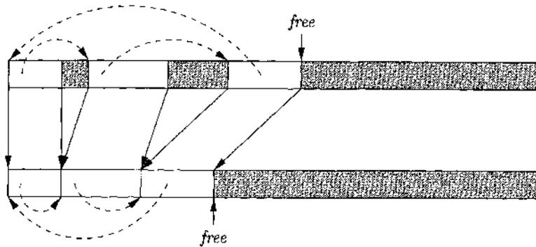
Figure 7.27: Moving reached objects to the front of the heap, while preserving internal pointers
