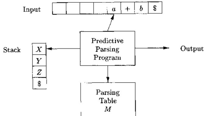
Figure 4.19: Model of a table-driven predictive parser
