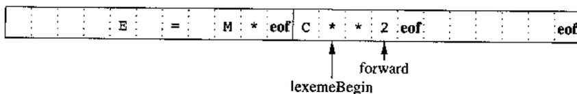
Figure 3.4: Sentinels at the end of each buffer
