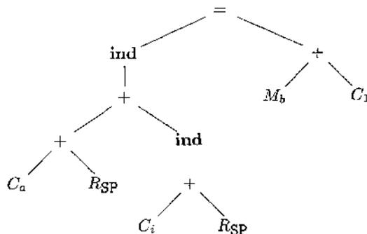
Figure 8.19: Intermediate-code tree for  $a[i] = b + 1$
