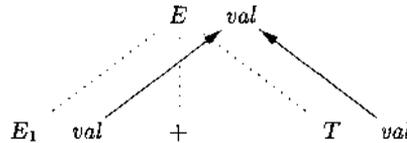
Figure 5.6:  $E.val$  is synthesized from  $E_1.val$  and  $E_2.val$
