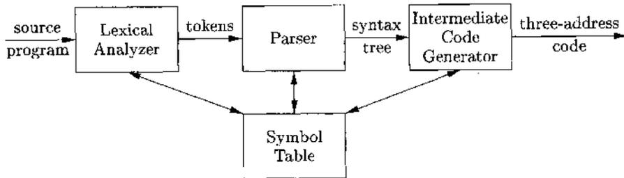
Figure 2.3: A model of a compiler front end
