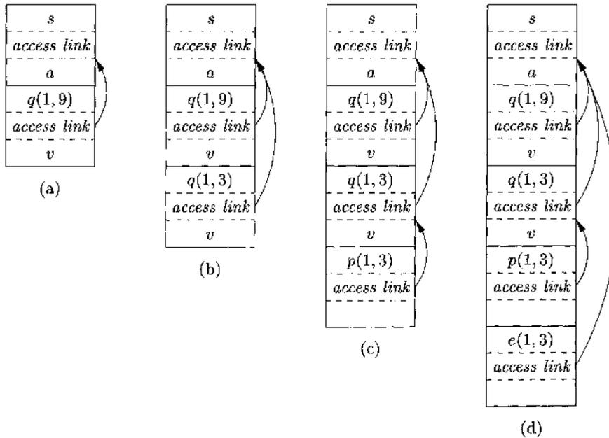
Figure 7.11: Access links for finding nonlocal data
