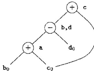
Figure 8.12: DAG for basic block in Example 8.10
