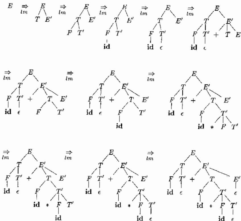
Figure 4.12: Top-down parse for  $\text{id} + \text{id} * \text{id}$
