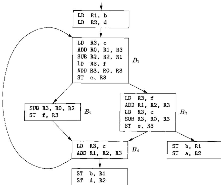
Figure 8.18: Code sequence using global register assignment
