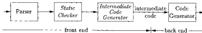
Figure 6.1: Logical structure of a compiler front end
