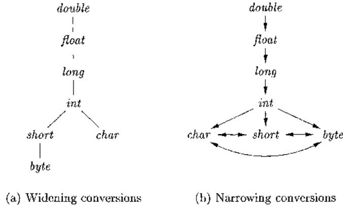
Figure 6.25: Conversions between primitive types in Java
