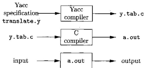
Figure 4.57: Creating an input/output translator with Yacc
