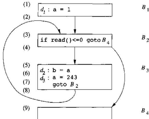
Figure 9.12: Example program illustrating the data-flow abstraction
