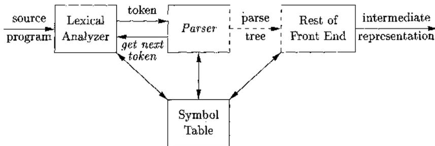
Figure 4.1: Position of parser in compiler model
