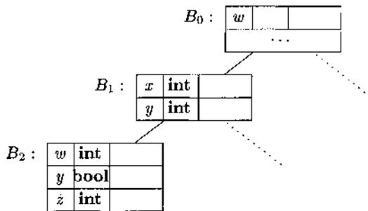
Figure 2.36: Chained symbol tables for Example 2.15
