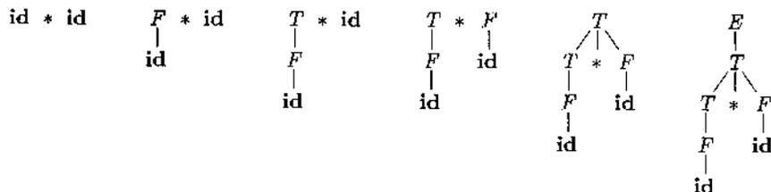
Figure 4.25: A bottom-up parse for  $\text{id} * \text{id}$
