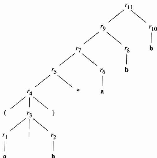
Figure 3.43: Parse tree for  $(a|b)^*abb$
