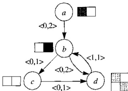
Figure 10.27: Dependence graph and resource requirement in Example 10.20
